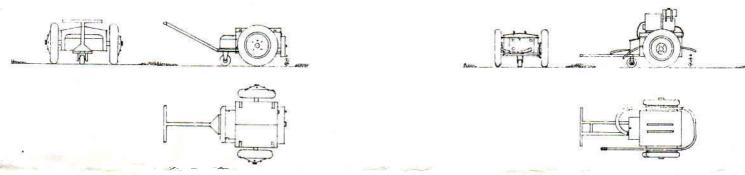
The trolley accumulator shown on the left was introduced into service in 1938 and continued in service well into the 1950s.
