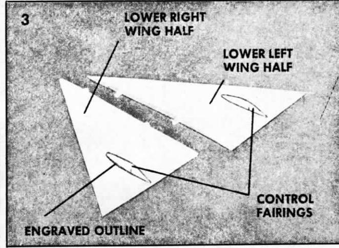
Glue the control fairings to the lower halves of the wings at the positions indicated by the engraved outlines.
