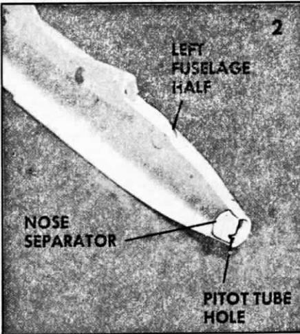
Glue the nose separator to the nose of the left fuselage half as shown. Note that the pitot tube hole is at the bottom.
