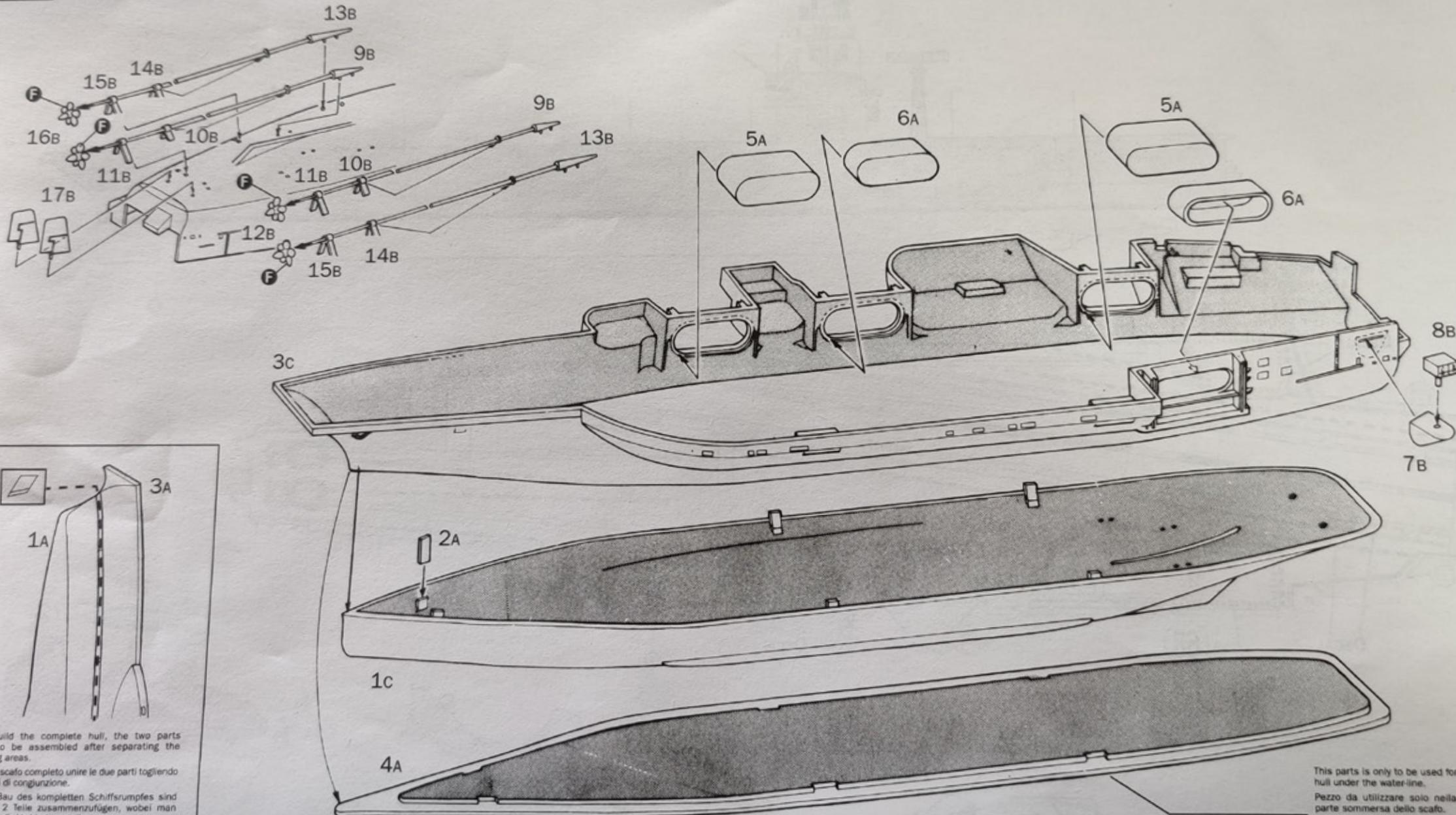
To build the complete hull, the two parts are to be assembled after separating the joining areas.
