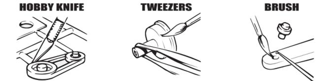
**HOBBY KNIFE:** Use a sharp hobby knife to remove parts from the trees. The knife may also be used to remove parting lines and flash.
