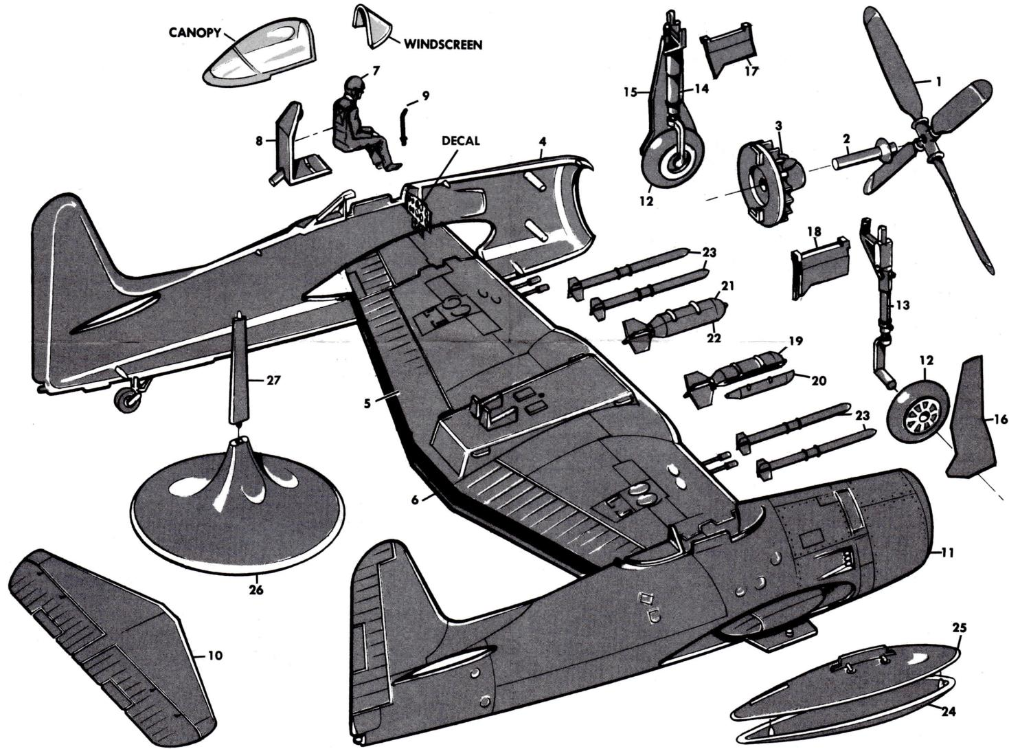
**1** Cement propeller 1 to short end of propeller shaft 2. Slip propeller shaft through hole in motor 3 and flare over end of shaft with the heated blade of an old knife. Cement backside of motor to pins in left fuselage half 4. Cut instrument panel from decal sheet and cement into left fuselage half.
