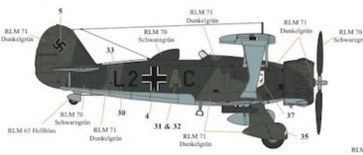
Hs 123 B-1 W.Nr 943 of 10.(Schl.)/LG 2 during the Balkan's campaign. Aircraft is in the simplified RLM 71 over 65 with RLM 04 tactical markings and revised dimension fuselage and lower wing crosses. Luftwaffe Im Focus No.17, p.13
