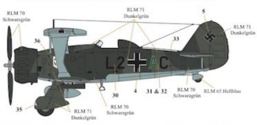
The photograph is poor quality but it can be seen that the aircraft has the new RLM 70/71 splinter scheme. Badge on left appears 'airbrushed' off photo but on most other photos from this unit the badge is on both sides. 'A' on wheel spats is speculative but not without president given the aircraft's other high viz markings
