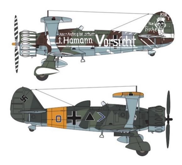
For the best results these decals should be applied to a gloss surface such as provided by either Xtracolor or Xtracrylix paints. Cut out the decal required and soak in warm water until the decal is released from the backing paper. Wet the area to be decaled with MICRO SET which will help to eliminate air trapped under the decal and position the decal.
