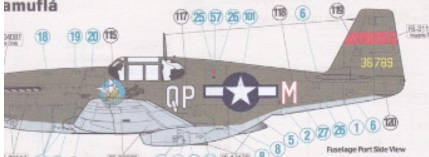
■ Airplane s/n 43-8789 Standard USAAF Olive Drab uppersurfaces and fuselage sides over Neutral Grey undersurfaces.
