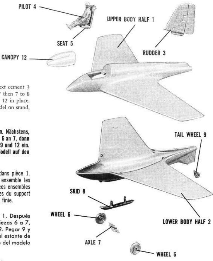
Cement parts 4 and 5 together then into part 1. Next cement 3 to 1 then 1 and 2 together. Cement both parts 6 to 7 then 7 to 8 and finally cement this assembly to 2. Cement 9 and 12 in place. Cement stand parts 10 and 11 together and place model on stand, see finished picture.
