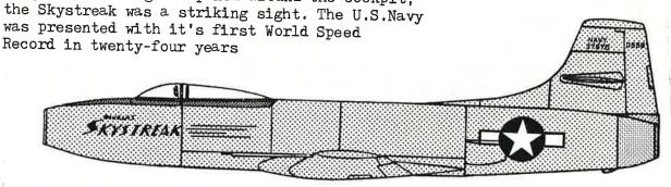
on August 20, 1947 when Cdr. Turner Caldwell took the first Skystreak 640.663 mph over a closed course. Five days later USMC Mjr.Marion Carl upped the record to 650.606 mph in the same aircraft. Both records were acheived with wingtip fuel tanks in place.
