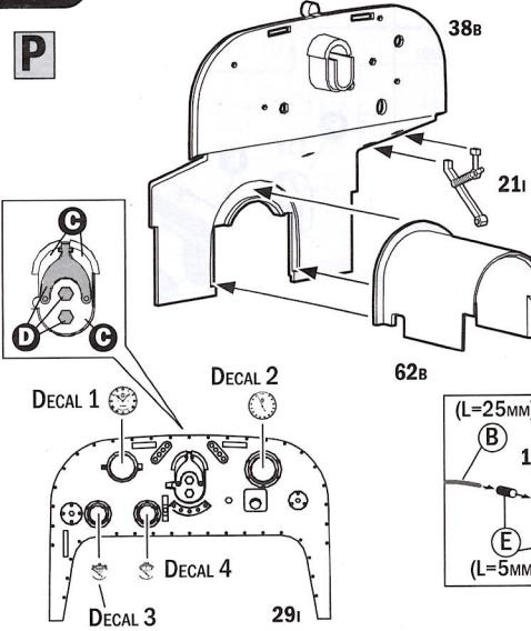
TUCK ALL MAGNETO WIRES (E) FROM THE PINS ON THE DASH INTO THE CENTER SLOT IN THE REAR PANEL AS WELL AS THE ANALOG INSTRUMENT WIRES
