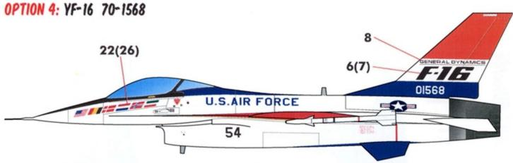
PAINT SCHEME AND STENCILLING GENERALLY IDENTICAL TO THAT OF OPTION I NOTE MISSING STENCILS IN THE NOSE AREA WHERE THE FLAGS WERE APPLIED
