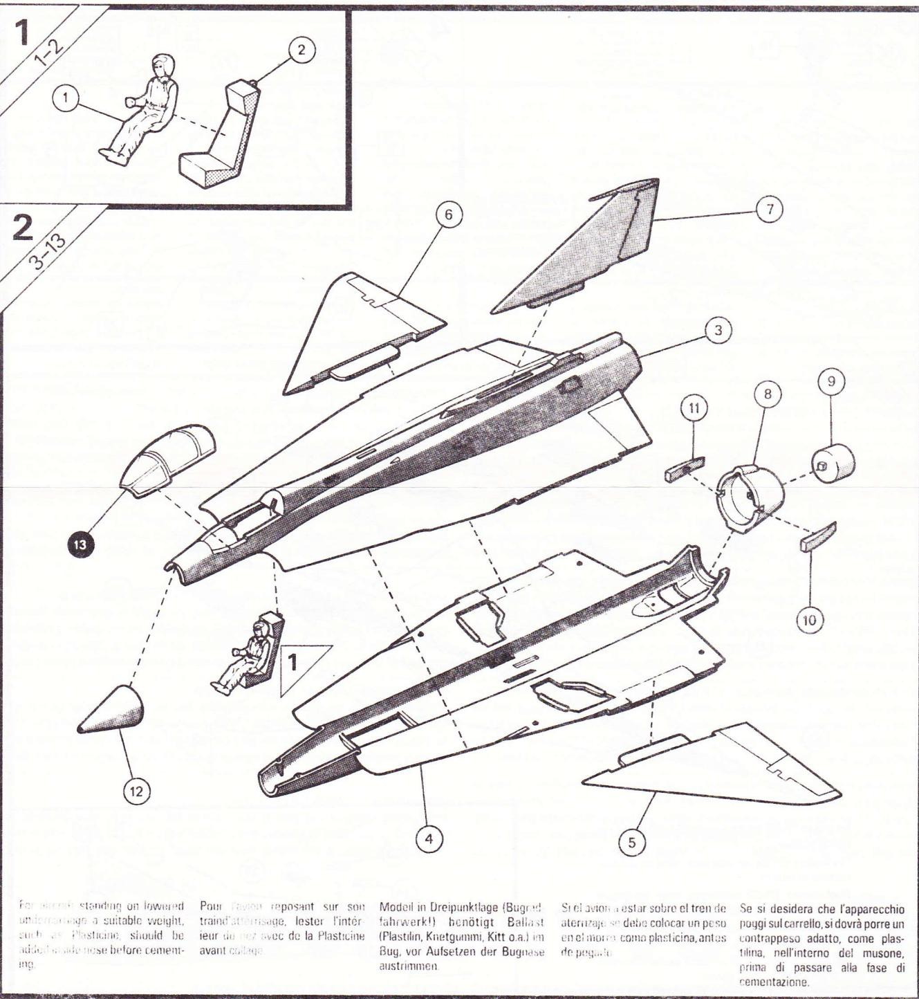
For success standing on lowered undercarriage a suitable weight, such as Plasticine, should be added inside nose before cementing.
