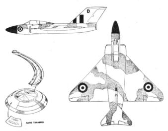
The Javelin was the world's first twin-jet delta fighter and was designed as a two-seat all-weather fighter. Our model is of the fourth prototype which was the first Javelin to be fitted with the double taper leading edge wing. The first prototype was flown on 26th November. 1951.
